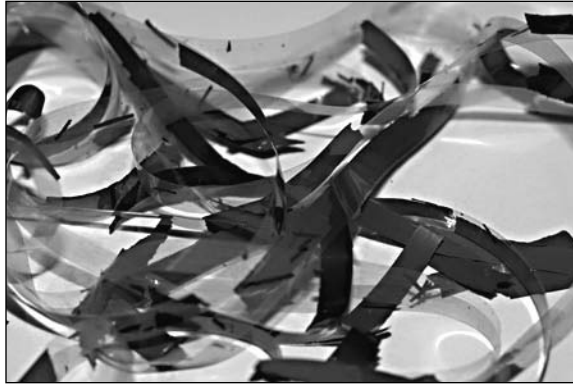
Figure 12. Binder-base adhesion failure (BBAF): A dual-layer Ferrochrome Type III cassette with an unknown and presumed-to-be-poor storage history. Source: the author.
