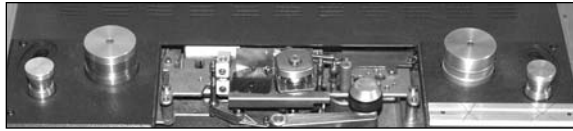
Figure 10. Controlling tape tension: A reel of Melody 169 that was recently transferred was done with a modified Studer A810 with the erase and record heads as well as some guides removed. Source: the author.
