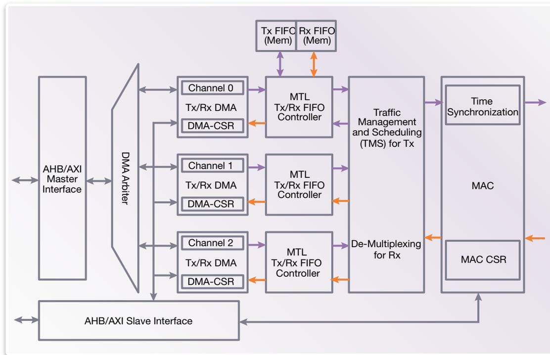
Figure 10: Top level block diagram of DesignWare ethernet QOS for AVB
