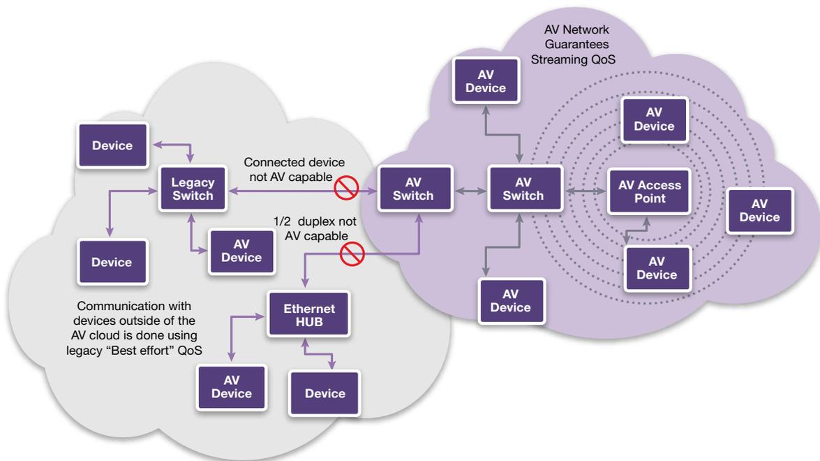
Figure 5: AVB network connected to legacy network
