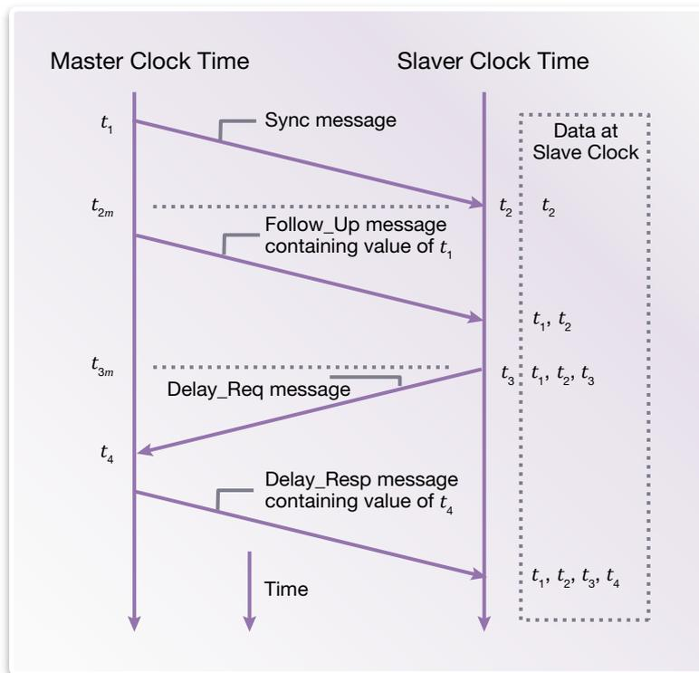
**Figure 6: PTP synchronization between master and slave nodes**
