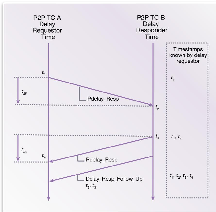
**Figure 7: Propagation delay calculation in clocks supporting peer-to-peer path correction**
