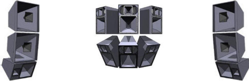
To produce the sounds from this center channel, we will need to provide a third set of loudspeakers to cope with it, although as typically the center channel is used for vocals, this third set of loudspeakers may not need the full range of drivers that the music channels normally utilise. For example, a sub-bass driver would be fairly ineffective on vocals as they do not reach such low frequencies.
