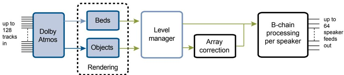
Figure 2.3 Block Diagram of Dolby Atmos Rendering
