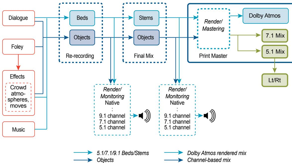
Figure 3.1 Dolby Atmos Audio Post Workflow
