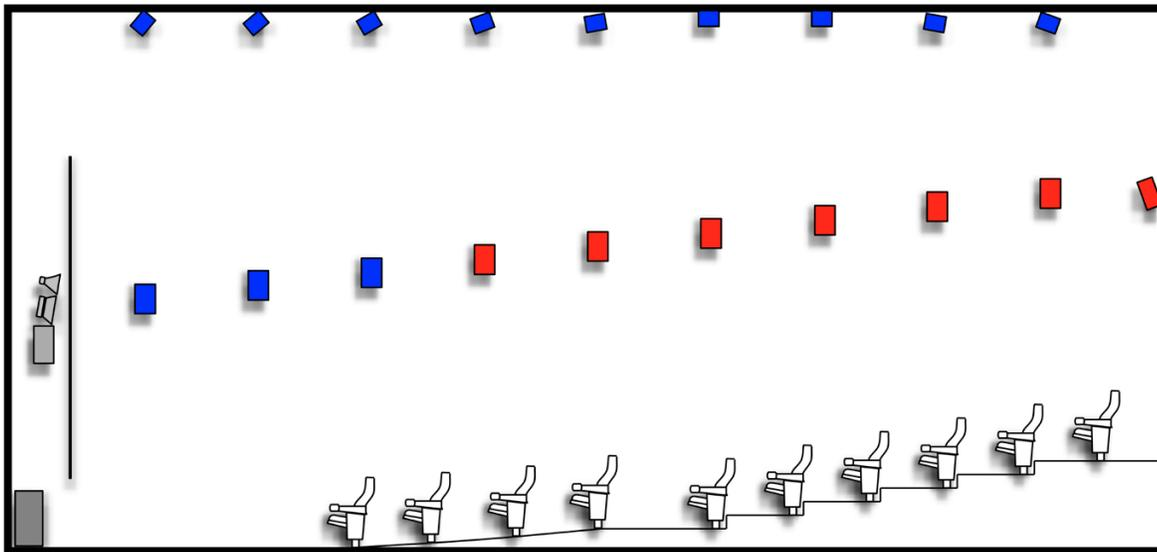
Figure 5.3 Recommended Side Wall and Ceiling Speaker Locations
