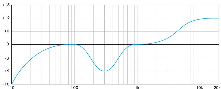
The term **Q** relates directly to the bandwidth of a bandpass filter. At a simple level it describes the ratio of the center frequency to the bandwidth.
