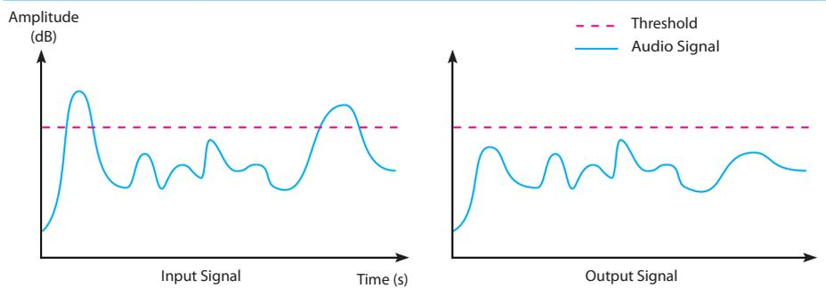
**FIGURE 6 - LOW THRESHOLD, LOW RATIO, WITH MAKE-UP GAIN**
