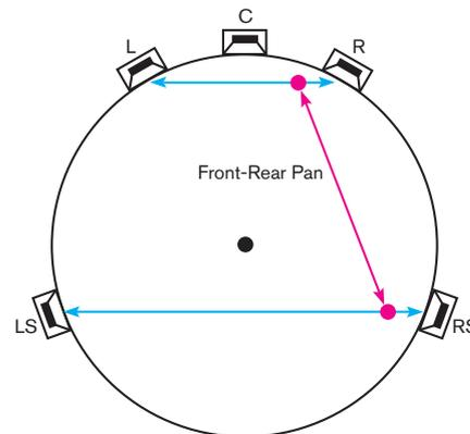
the center's contribution to L and R. A full divergence value means that no signal is present in the center, and is split fully between L and R. See Figure 3 for an illustration of this process.
