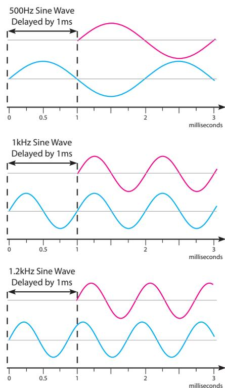
consider there are two identical signals, each made up of a 1kHz sine wave and a 650Hz sine wave. If the 650Hz component of the first wave is delayed, the 650Hz components of both waves are out of phase but the 1kHz components are still in phase.
