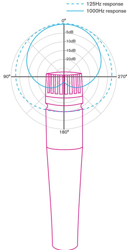
A reverse version of the plot shown here can be used, for example when working with loudspeakers. In this situation the plot would show the level of signal the device would emit in all directions at a certain frequency.
