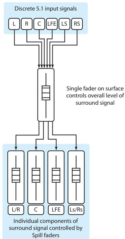
attached to whichever fader is currently assigned on the surface. If a different fader is assigned, the Spill panel will update to reflect the state of the signal attached to this newly assigned fader.
