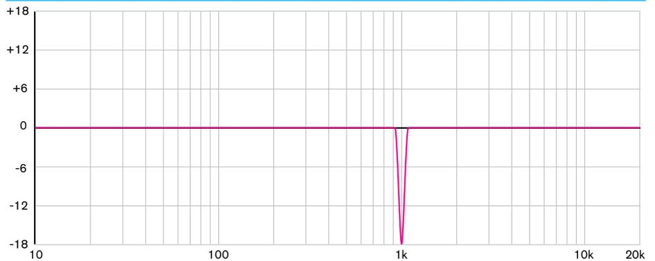
Common uses include removing the high frequency whistle produced by CRT television sets, or removing problematic resonant frequencies.
