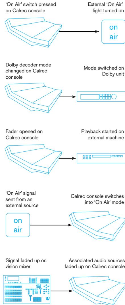
Setting the output to 'Pulse' opens the relay for a duration of 100ms then closes it. The relay can be set to pulse when the control message is activated, de-activated or both.
