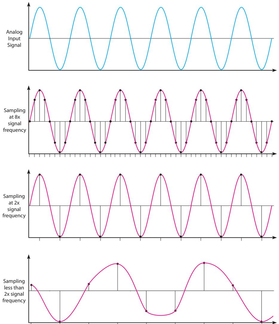
In a digital system the incoming continuous signal is periodically sampled, each sample having a discrete value. This means that for any given sample at any time interval, a definite value can be retrieved at any time and the value and accuracy of that sample will always be the same no matter when it is retrieved.
