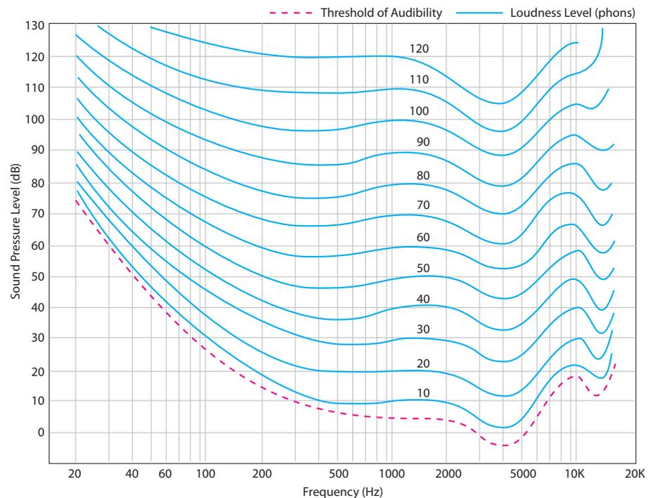
had created an audio mix at high listening levels and decided that the overall spectral balance was as desired. You may find that when played back on a system at a lower listening level, the mix may be lacking in low and high end detail compared with other successful mixes.
