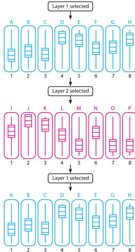
Paths assigned to layers that are not visible on the surface will still pass audio through the console. They cannot be controlled manually directly unless they are assigned to faders and present on the surface.
