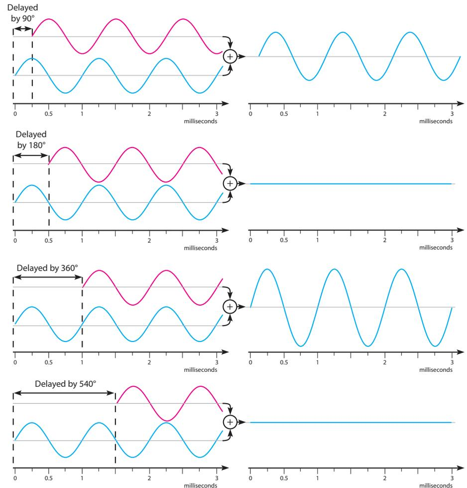
Because the red wave is being delayed by a degree value, which relates directly to a position in the cycle, the frequency of the waves is irrelevant. As long as they are both the same, these waves could be of any frequency and the results would remain the same.
