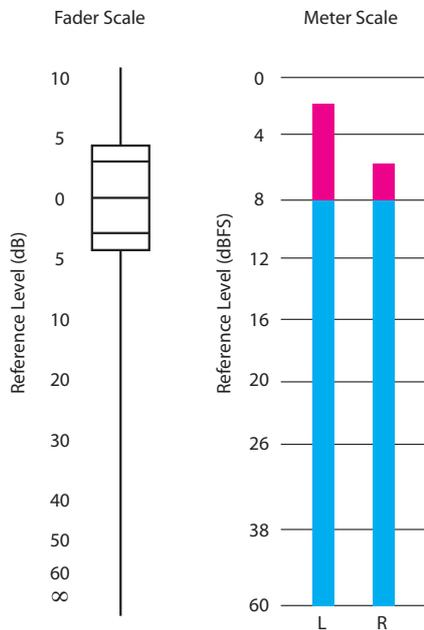
In this case the dB ratio will not refer to sound pressure level, but to a generic dB ratio.
