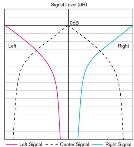
is panned between the center speaker and the left or right speaker. Looking at Figure 3 it can be seen that as the signal is panned right of center, the left speaker receives no signal at all.
