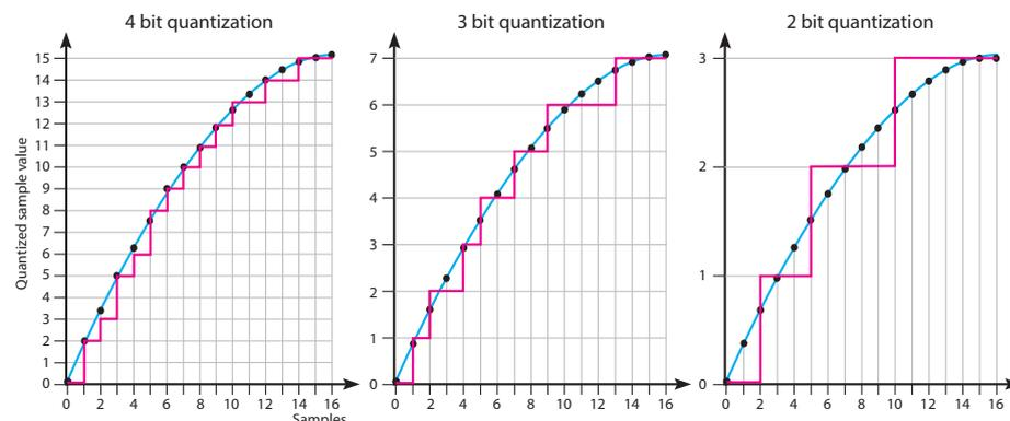
is determined by the bit depth of the digital signal.
