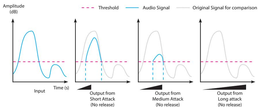
transition. A long attack time produces a smoother fade transition but will lose some transient information. Figure 3 shows a representation of some of attack parameters. The black triangles below each graph show the duration of the attack, and the level of the audio signal (from maximum attenuation to original strength).
