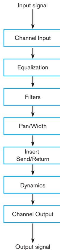
**FIGURE 2 - INSERT SIGNAL FLOW**
