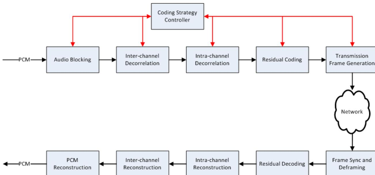
**Figure 1: apt-X Lossless Conceptual Architecture**
