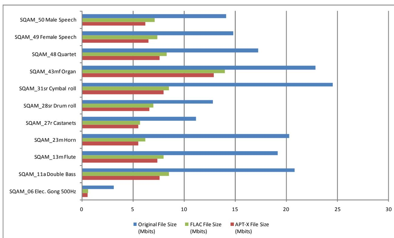
**Figure 2 : apt-X Lossless Performance Example**
