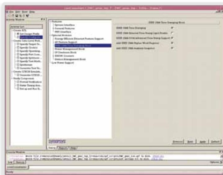
Figure 9: DesignWare ethernet QoS IEEE 1588-2008 configuration menu
