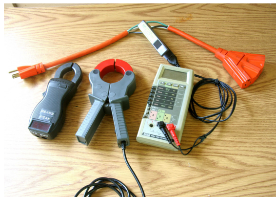
Fig 20 – Current probes and breakout cable
