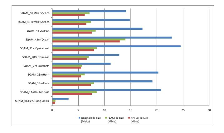
Figure 2 : apt-X Lossless Performance Example
