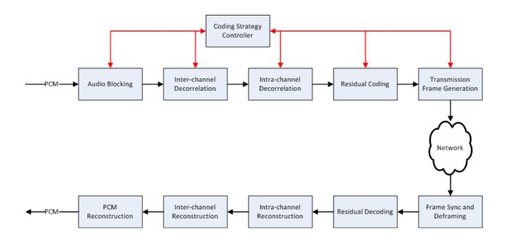
Figure 1: apt-X Lossless Conceptual Architecture
