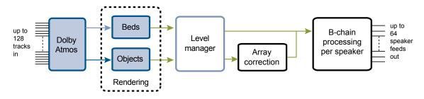
Figure 2.3 Block Diagram of Dolby Atmos Rendering
